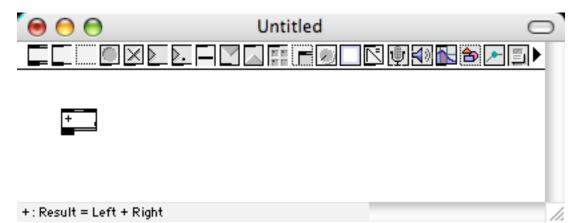
There are two modes of patch cord entry. If "Segmented Patch Cords" is not checked in the options menu, you must drag a cord directly from an outlet to an inlet to make the connection. If the option is checked, clicking on a outlet will start the cord, and clicking in empty space will put a corner in the cord. Click on an inlet to finish the connection If you find a cord stuck to the mouse with nowhere to put it, command click on empty space.
